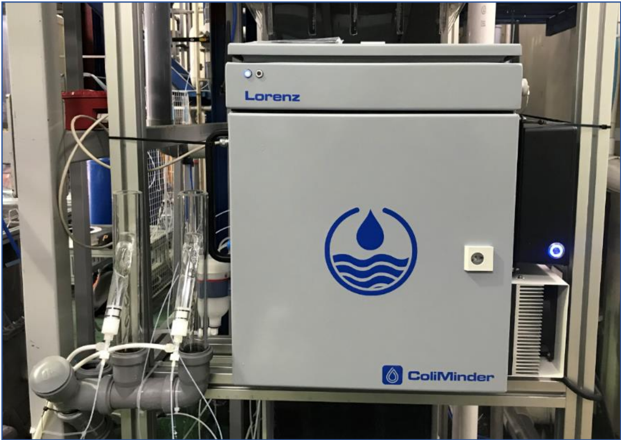
FIGURE 1: COLIMINDER “LORENZ” EQUIPPED WITH TWO SAMPLING UNITS AT SEOUL METROPOLITAN WATER INSTITUTE
